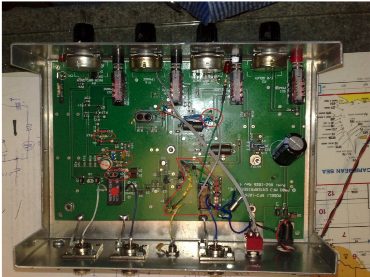
Figure 4 - The signs in red represent the changed areas. In line with the coaxial connector (AUX) at the bottom right is the additional protection circuit and the relay RL1a is visible; this circuit is active both with PTT command and with RF detection and automatic switching. Next to the connector is the switch associated with the Phase Extension, located in place of the RCA antenna socket.
